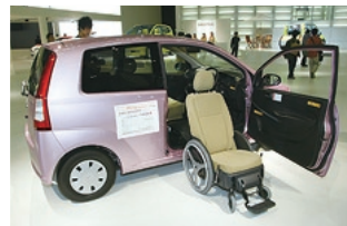
The Mira Selfmatic is designed to be driven by the physically-challenged
