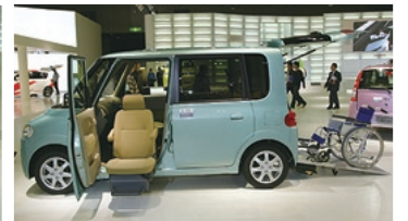
The Mira Selfmatic is designed to be driven by the physically-challenged
