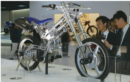
The electric DEINONYCHUS with in-wheel, two-wheel drive
