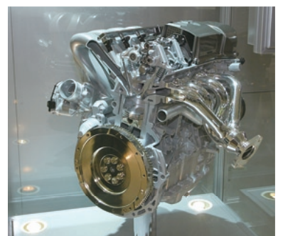
The cutaway model of the MIVEC engine in the technology zone
